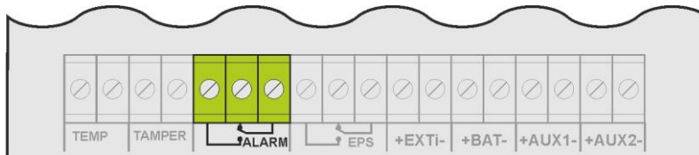
Fig. 9. Technical output ALARM.
