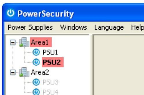
Fig. 6. Status indication of the monitored power supplies.
